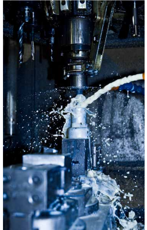
Machining of the pump cylinder in our CNC machining centre
