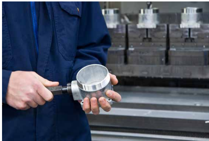
Quality control of the connecting flange after machining
