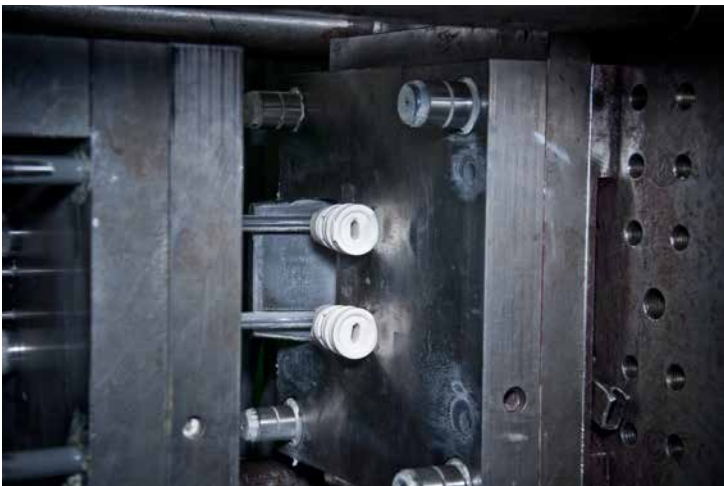
Plastic injection molding of the distributor
